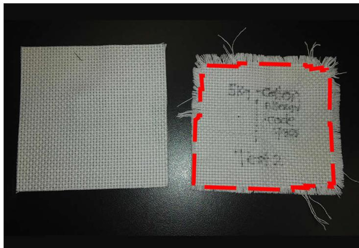
**Figure 2:** Gentleness of action (fray) swatches- before and after wash cycle
