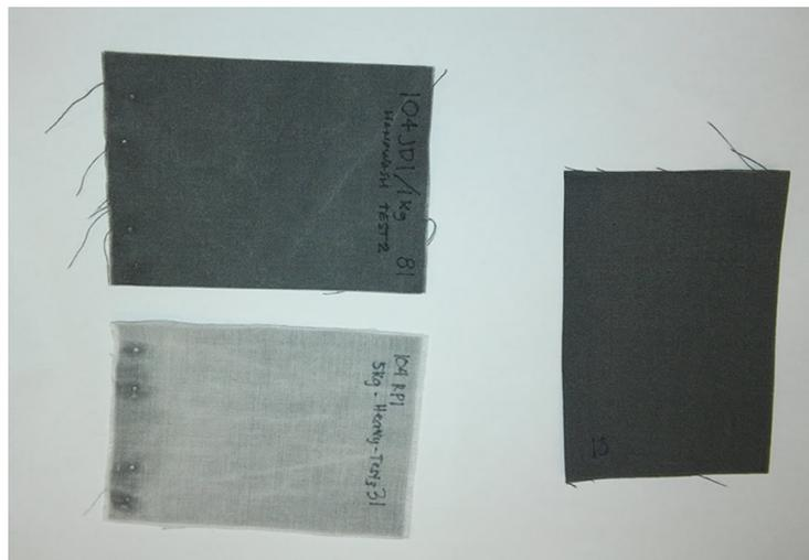
**Figure 1:** Soil removal swatches, before and after wash cycle (top was heavy cycle; bottom was delicate cycle)
