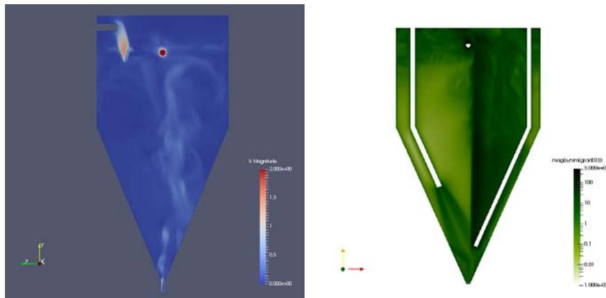
Figure: (Left) Flow velocity of original large tank. (Right) New design of large tank, with water and air supplied at the bottom
